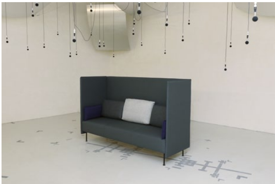
Series Creva soft – tested in the reverberation chamber in compliance with DIN EN ISO 354:2003
